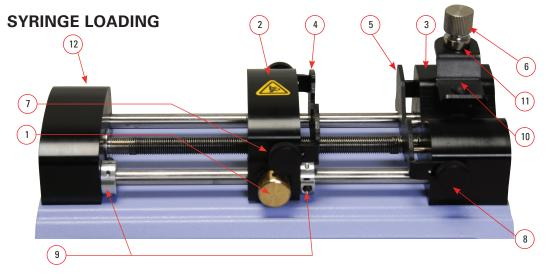
The Pump 11 Elite Series can accommodate up to two syringes. Depending on the mechanism, any type of syringe, glass, plastic or stainless steel can be used. The Pump 11 Elite can accommodate from  $0.5~\mu l$  to 60 ml single syringe and  $0.5~\mu l$  to 10 ml dual syringe. The syringe barrel clamp should be flipped for syringes smaller than 30 ml. For syringes larger than 30 ml the syringe clamp should be used as shown.
