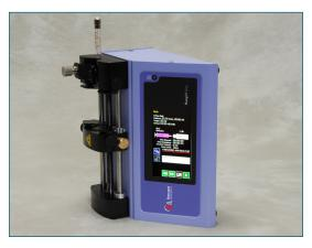
Advanced microstepping techniques are employed to further reduce the step angle to eliminate flow pulsation. The accuracy is 0.5% (0.35% for Pico Plus Elite). A wide dynamic flow range from 1.26 pl/min to 88.40 ml/min (0.54 pl/min to 11.70 ml/min for the Pico Plus Elite) can be programmed into the pump. Flow rates are selectable with user selected engineering units from ml, µl, nl, pl, and hours, minutes and seconds.
