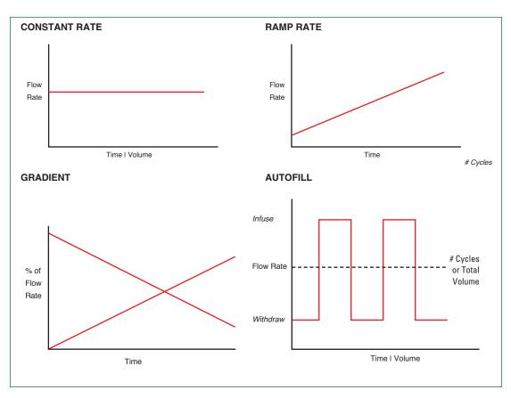
**Pump Operation Profiles available on the Pump 11 Elite Series**
